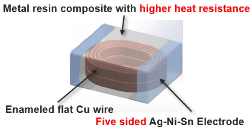
Figure 5. ME series inductor's construction
