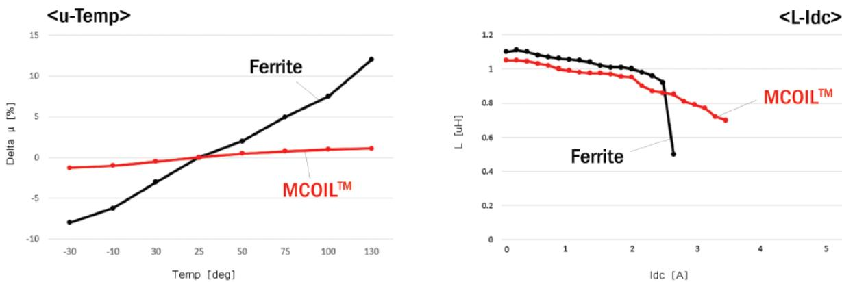
Figure 6. MC series inductor's inductance stability versus ferrite
