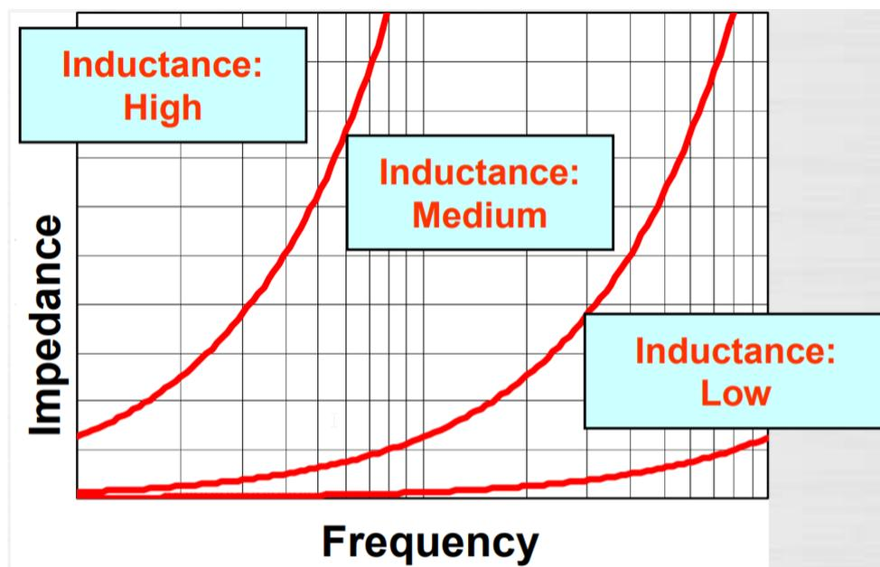
Figure 2. Typical impedance vs frequency curves for inductors<sup>2</sup>
