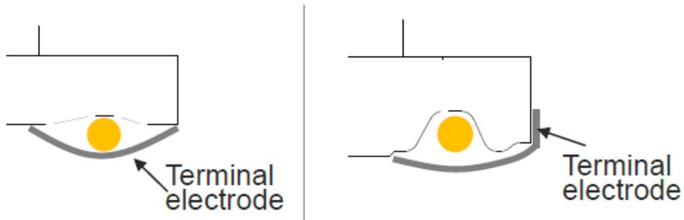
Figure 4. Traditional electrode structure versus NR series M-type's side terminals
