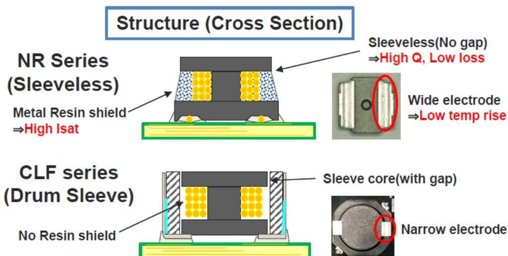
Figure 3. Sleeveless inductor cross section versus alternative
